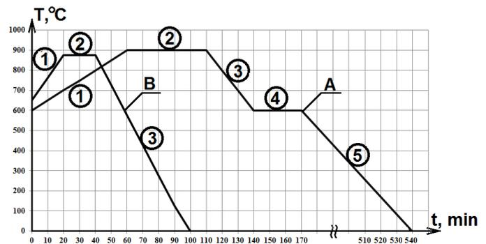
Figure 3. The optimum temperature-time modes of block (A) and granulated (B) FSG synthesis: 1 - calefaction, 2 - foaming, 3 - rapid cooling with porous structure stabilization, 4 additional stabilization, 5 - gradual cooling – annealing
