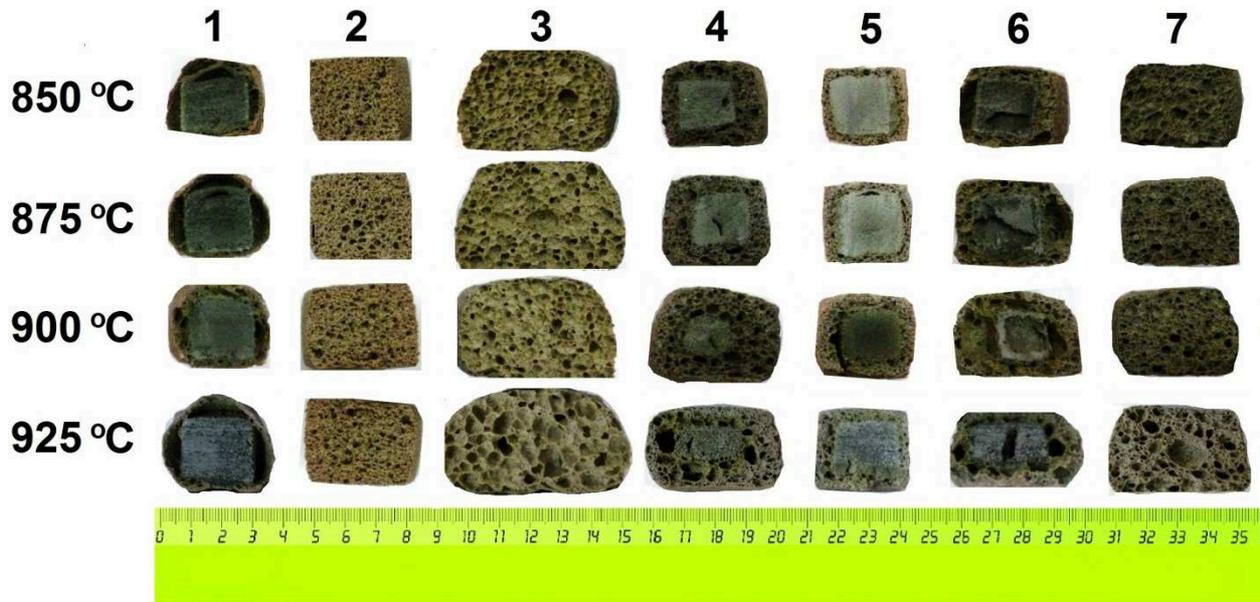
Fig. 3. Influence of the type and amount of foaming agents on the structure of foamed slag glass
