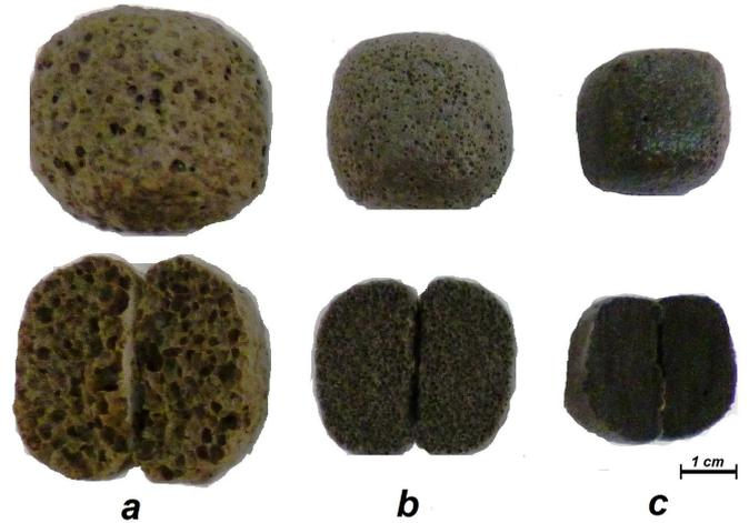
Fig. 3. Foam glass based on various glasses.
