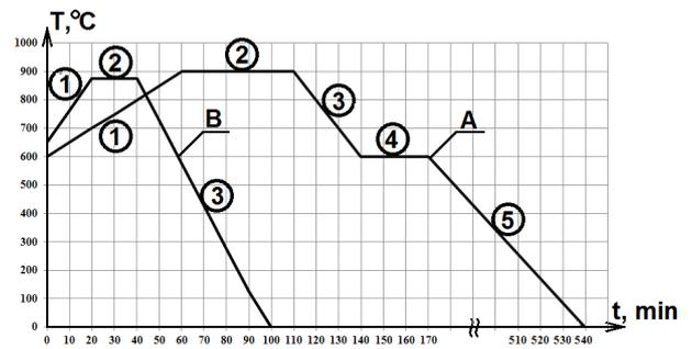
Fig. 7. The optimum temperature-time modes of block (A) and granulated (B) FSG synthesis: 1 - calesfaction, 2 – foaming, 3 – quenching (rapid cooling) with structure stabilization, 4 – additional thermal stabilization, 5 – annealing (gradual cooling).
