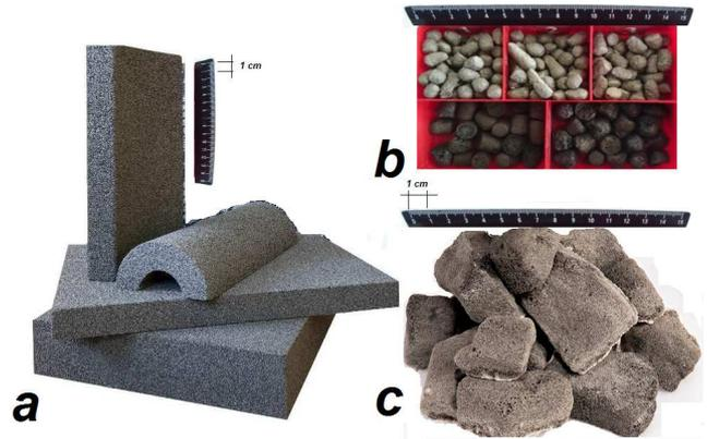
Fig. 8. FSG-based products: a – blocks, b – granules, c - breakstone.
