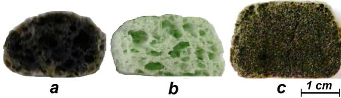
Fig. 4. Foam glass based on various foaming agents.
