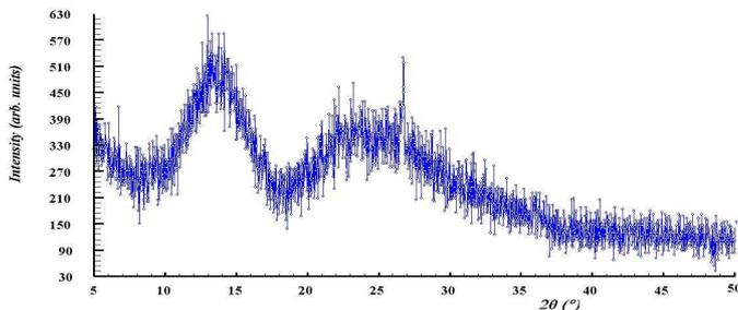
Fig. 5. X-ray analysis of slag waste.
