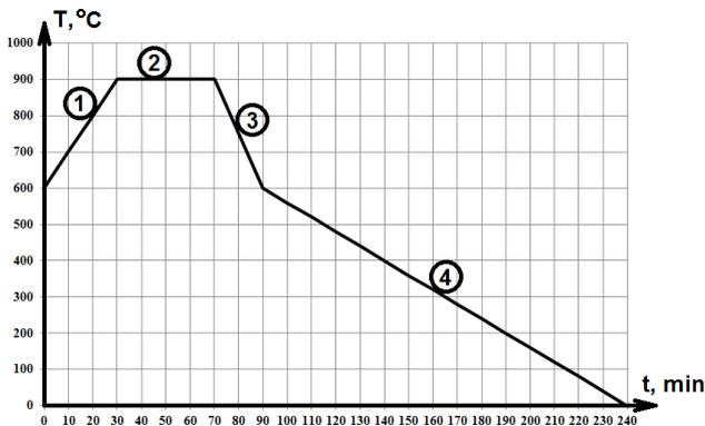
Fig. 2. Foam glass synthesis schedule: 1 - calefaction, 2 - foaming, 3 - quenching (rapid cooling) with structure stabilization, 4 - annealing (gradual cooling).
