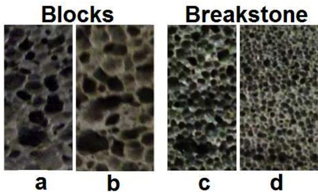
Fig. 9. Photographs of macrostructure of obtained materials in comparison with market counterparts: a - «Gomelglass» foam glass block; b – FSG block; c – «ICM Glass Kaluga» foam glass breakstone; d – FSG breakstone.
