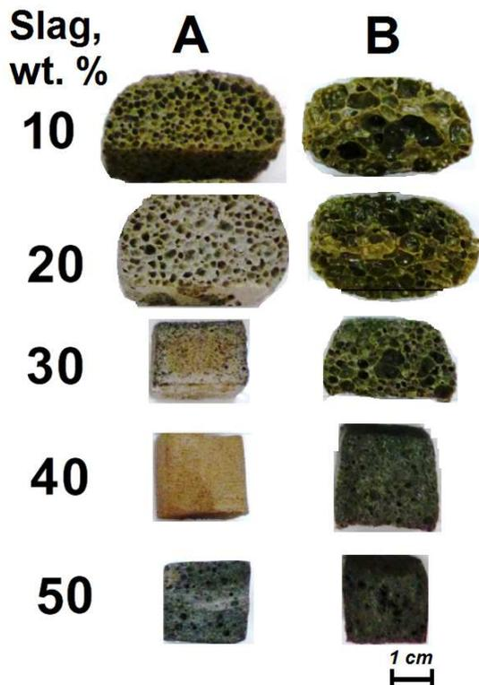
Fig. 6. Foamed slag glass with various content of slag.
