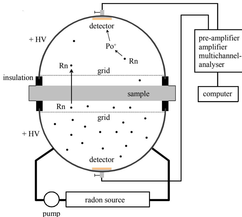
Figure 1. Principle of the measuring method for determining the radon diffusion coefficient
