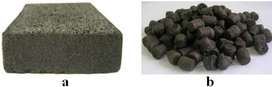
Figure 8 – Appearance Designs of block (a) and granulated (b) foamed slag glass.
