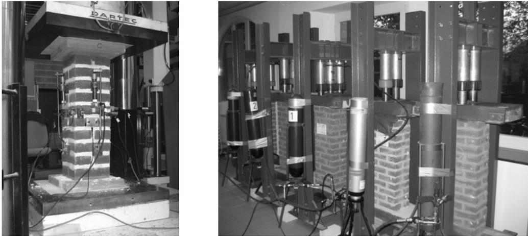
Fig. 3. Typical short-term (a) and long-term (b) creep test set-up
