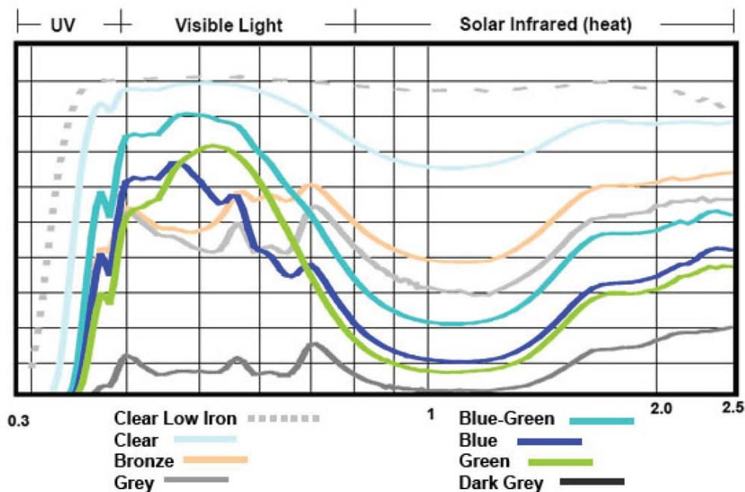
Figure 8. UV, visible, and near infrared transmission (300-2500 nm) of common glass with different colours. Arsenault, 2015.
