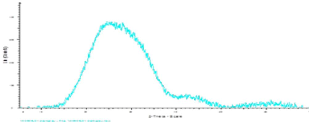
Figure 5. X-Ray Diffraction pattern of soda lime silicate glass. Due to the amorphous glass structure of the substance, no X-ray diffraction peaks appear. Horizontal axis:  $2\theta$ , vertical axis: intensity (counts).
