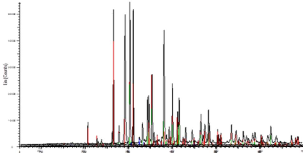
Figure 4. X-Ray Diffraction pattern of a mixture of sand (quartz), soda ash, limestone and dolomite. Horizontal axis:  $2\theta$ , vertical axis: intensity (counts).
