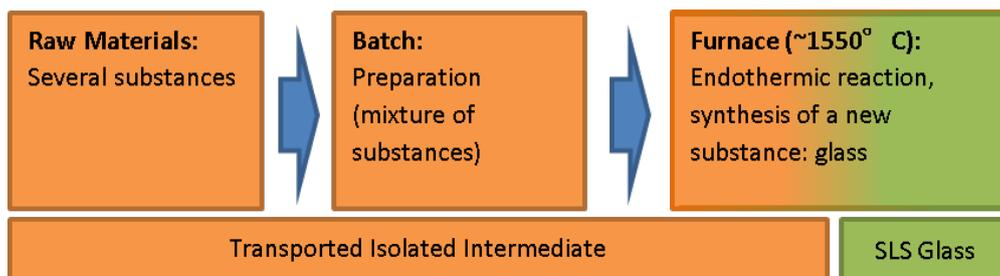
Figure 2. Formation of the substance SLS Glass from raw materials.
