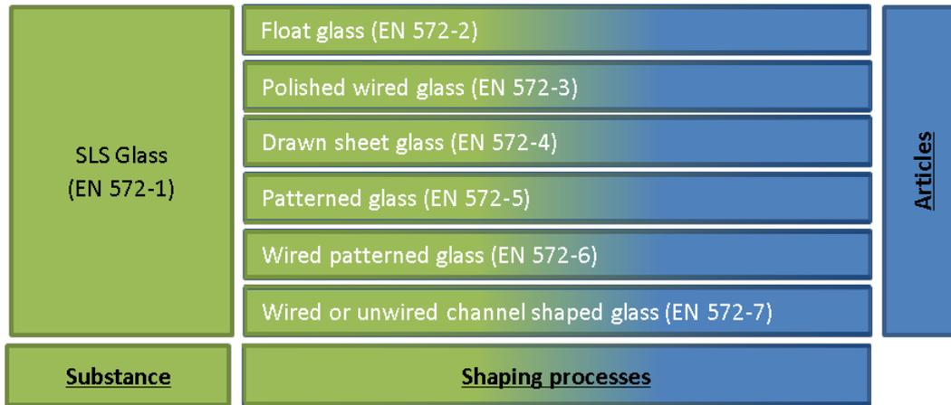
Figure 3. Shaping of the substance SLS glass into articles.
