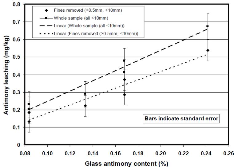
Figure 10. The relationship between glass composition and leaching. Average results of Sb leaching tests (EN 12547-4) on rolled plate glass for Photovoltaic panel cover. ICG TC13 document, 2010.
