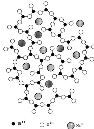
Figure 6. Glass structure showing the silicon tetrahedrons linked together to form the network. Larger ions such as  $\text{Na}^+$  are placed outside the tetrahedron. Zarzycki, 1982.
