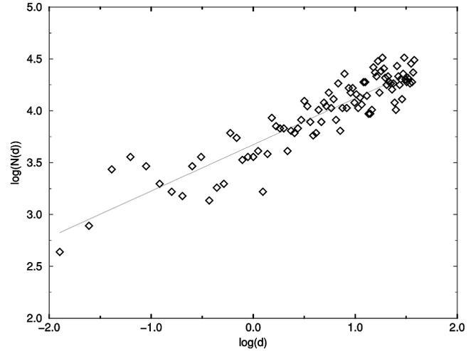
FIG. 4. Plot of the logarithm of the number of consecutive events at distance  $d$  versus the logarithm of  $d$ . This however is not the real (three-dimensional) distance but the distance ( $d^2 = x^2 + y^2$ ) after projection on a plane perpendicular to the stress. The experimental results (diamonds) are compared with a linear fit with slope  $0.4$ .
