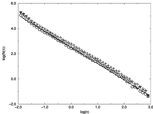
FIG. 3. The logarithm of the number of events registered with an interarrival time  $\tau$  (in s) is plotted versus the logarithm of  $\tau$ . This is done for three different loads (circles, triangles, and crosses). A linear fit of the experimental values gives slope  $-1.28$ ,  $-1.29$ , and  $-1.27$ .
