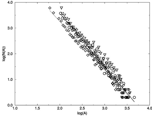
FIG. 2. The logarithm of the number of registered events with amplitude  $A$  is plotted versus the logarithm of  $A$  (in  $\mu\text{V}$ ) for three different loads (diamonds, triangles, and circles). The experimental results can be fit by a line with slope  $-1.90$ ,  $-2.10$ , and  $-2.08$ , respectively.
